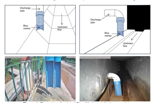
Figure 1. Examples of painted Blue-Marker at discharge points.
